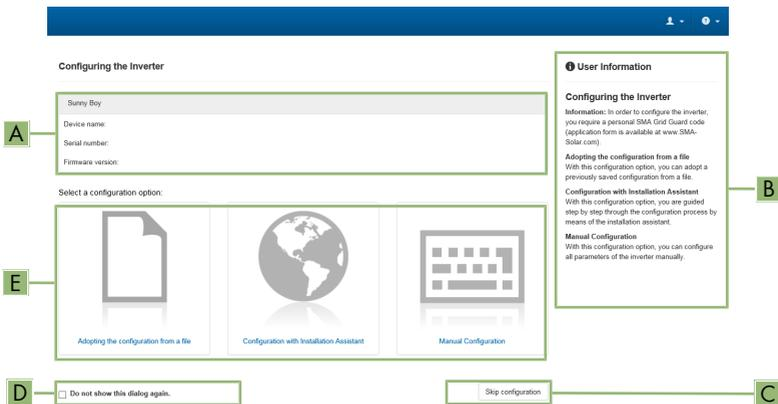
Figure 21: Layout of the **Configuring the Inverter** page
