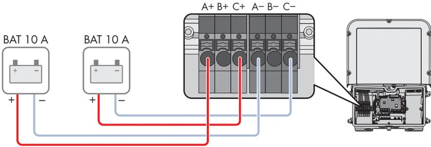
Figure 16: Overview for connection of two batteries with a charging/discharging current limit of 10 A each
