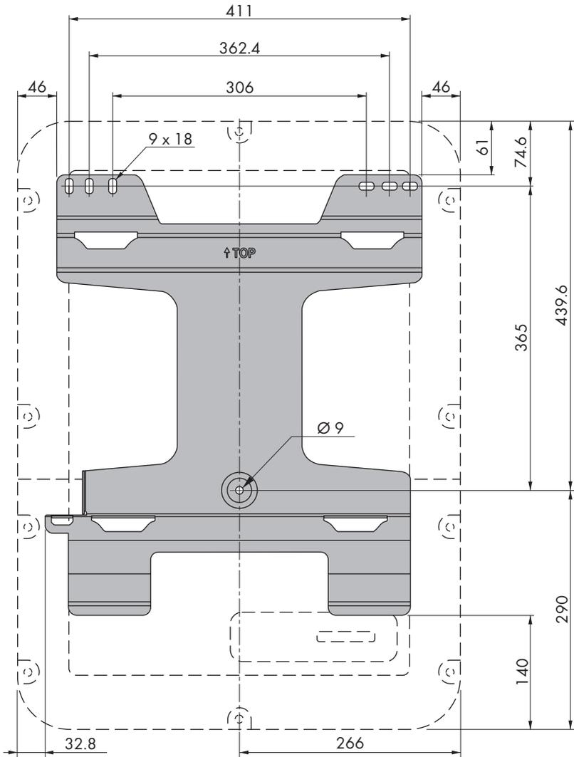
Figure 11: Position of the anchoring points(Dimensions in mm)
