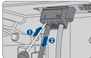
4. Screw out the screws from the **AC-out** terminal block using a flat-blade screwdriver (blade width: 3.5 mm) and pull the terminal block out of the slot.
