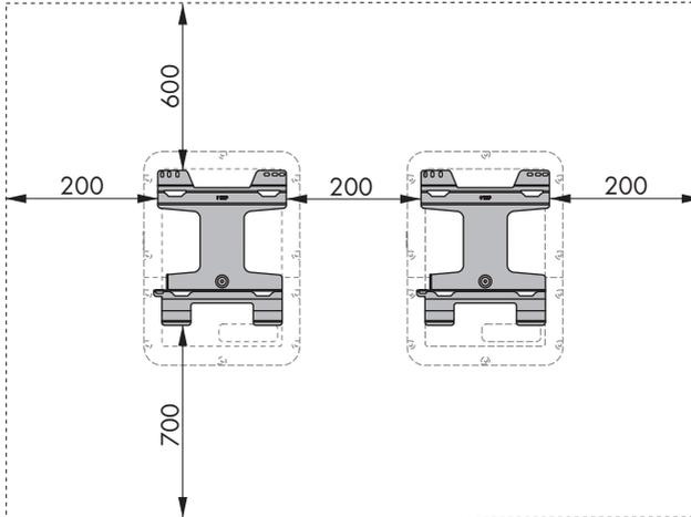
Figure 12: Recommended clearances (Dimensions in mm)
