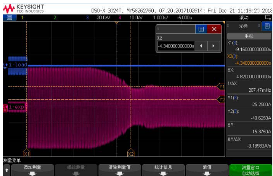
Test Category: Only the photovoltaic (PV) Reaction time: 4.82S
