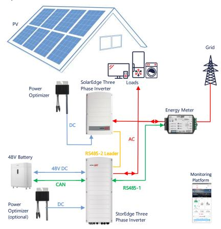
In addition to the AC-coupling, the StorEdge three phase inverter can also be equipped with PV power optimizers. In case there is no communication between the 2 inverters, in order to work in MSC mode, it is mandatory to connect production meter on the output of the existing inverter and connect its communication to the leader. Please refer to the user guide for detailed connection procedure.
