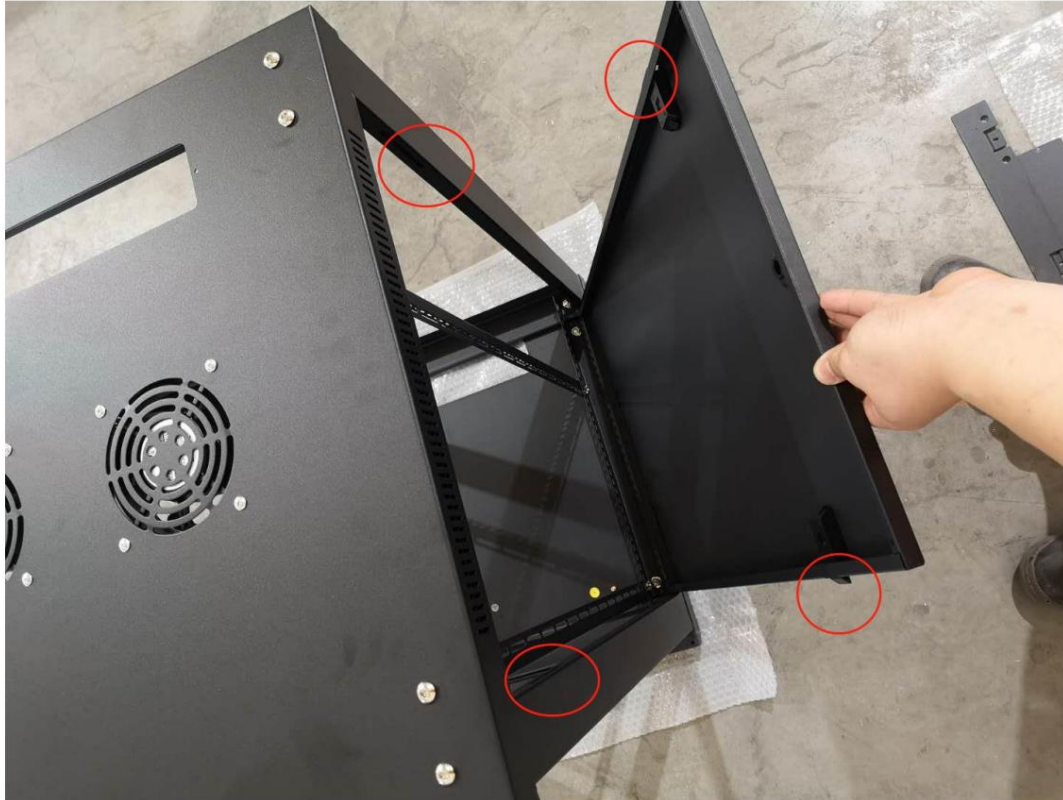
Placing the door is very intuitive, the important part is securing the slots for the door latch.
