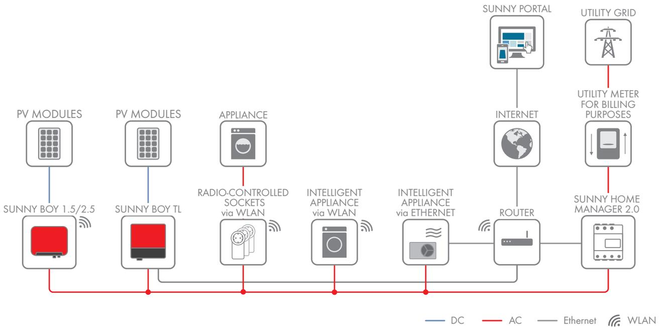
**PV system with inverters of other manufacturers and measurement at the grid-connection point and the PV generation using a Sunny Home Manager and an SMA Energy Meter**
