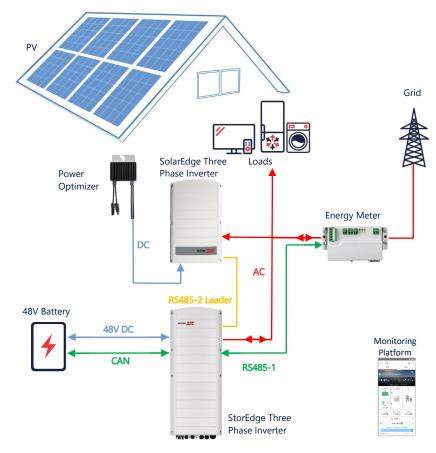
In addition to the AC-coupling, the StorEdge three phase inverter can also be equipped with PV power optimizers.
