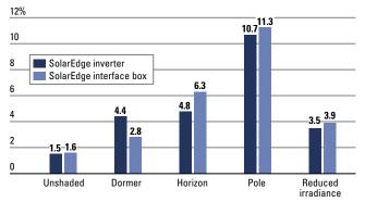
The additional yields produced by installing PowerBoxes with systems that have comparatively short strings are rather modest. But performance is greatly improved by the devices when a system is shaded by a pole.
