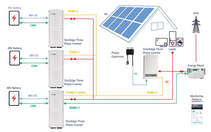
The up to three StorEdge Inverters can also have Power Optimizers or can be AC-Coupled to a non-SolarEdge power source, as explained in the below use case.
