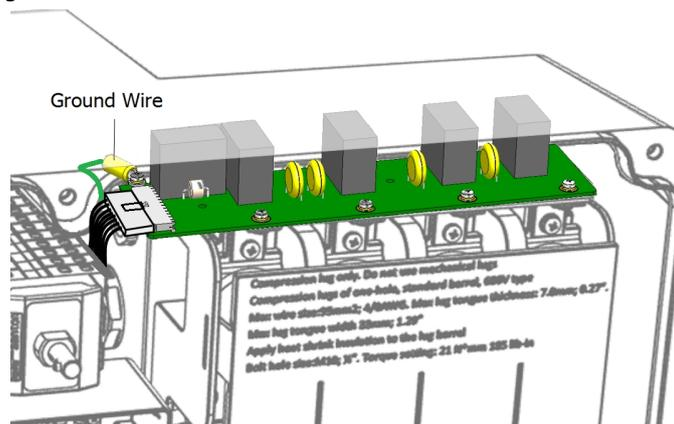
Figure 3: AC SPD Board Removal
