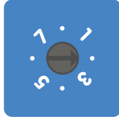
Rotary switch set to position 2
