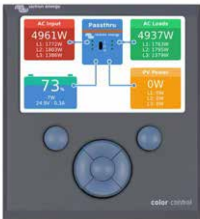
Color Control panel, showing a PV application
