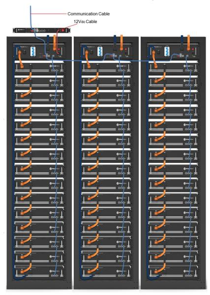
**Note:** The 1st PowerCube-H1/H2 should be installed nearest to the MBMS.
