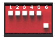
ADD Switch MBMS is a 6 bit dial switches to manually distribute the communication address of the battery system. Nether position is OFF, means "0". Upper position is ON, means "1". 1st bit to 4th bit is for address, the 5th and the 6th bit dial switch support a  $120\,\Omega$  resistance (**Terminal Resistance**).
