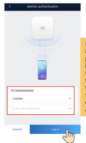
Log in to the app as an intaller. The initial password of the installer is 00000a. If the system prompts you to set a password, set the password and login first power-on and change it immediately after login.
