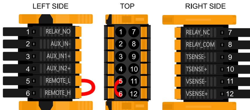
User I/O Connector is located on bottom left side of connection area, diagram shows 3 perspectives. Left Side - Top - Right Side
