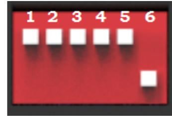
**ADD Switch MBMS** is a 6 bit dial switches to manually distribute the communication address of the battery system. Nether position is OFF, means "0". Upper position is ON, means "1". 1<sup>st</sup> bit to 4<sup>th</sup> bit is for address, the 5<sup>th</sup> and the 6<sup>th</sup> bit dial switch support a 120 Ω resistance (**Terminal Resistance**).
