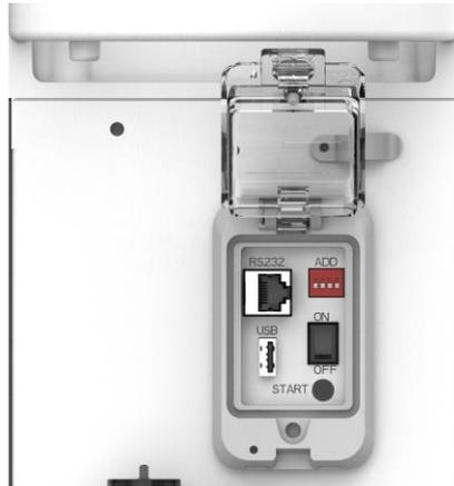
2) Press the **START button** for more than 3 second to power on, all the LED lights of battery modules will be white which means you launch it successfully. Then the rest batteries will start one by one and keep one light flashing after all the LED lights on.
