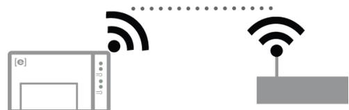
If you are not using the Installer Toolkit mobile app, you can only connect using WPS. Initiate a WPS connection by pressing and holding the **AP Mode** button for 5 seconds.
