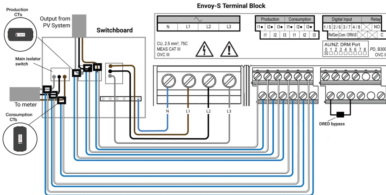
**Install the CT(s) for Production Metering**
