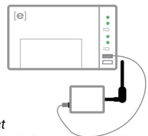
Within three minutes the Envoy-S Network Communications LED
