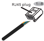
Figure 4.22 Strip the insulation layer and connect to RJ45 plug
