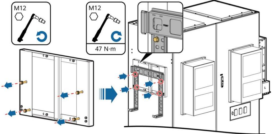
2. Install mounting ears and lifting handles, and then secure the Smart PCS. The mounting ears are delivered with the Smart PCS, and the lifting handles are delivered with the ESS.
