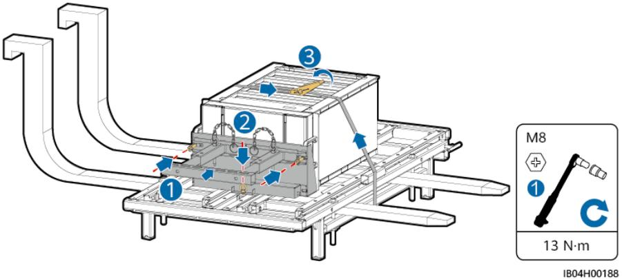
6. Move the forklift to the vicinity of the ESS, adjust the height of the installation kit, and remove the battery pack straps.
