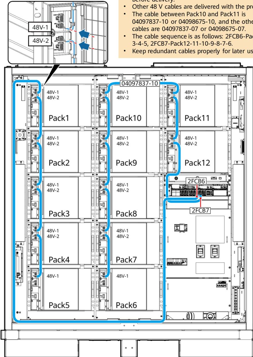
3. Install cables to the COM ports.
