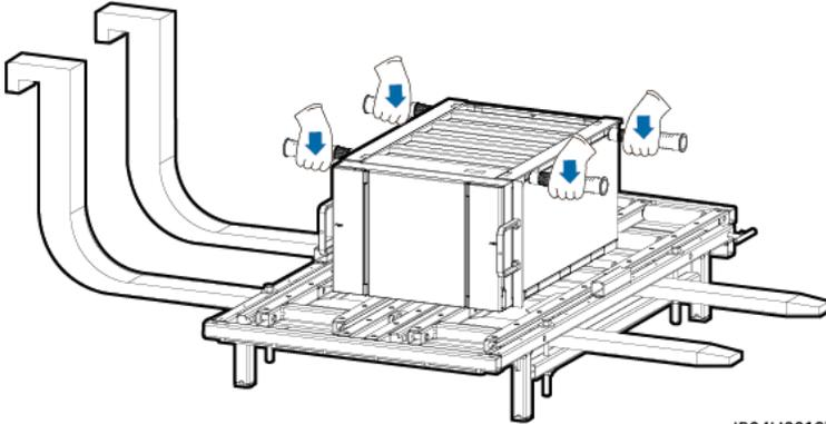
5. Install the shovel pan, positioning pin, and binding straps.
