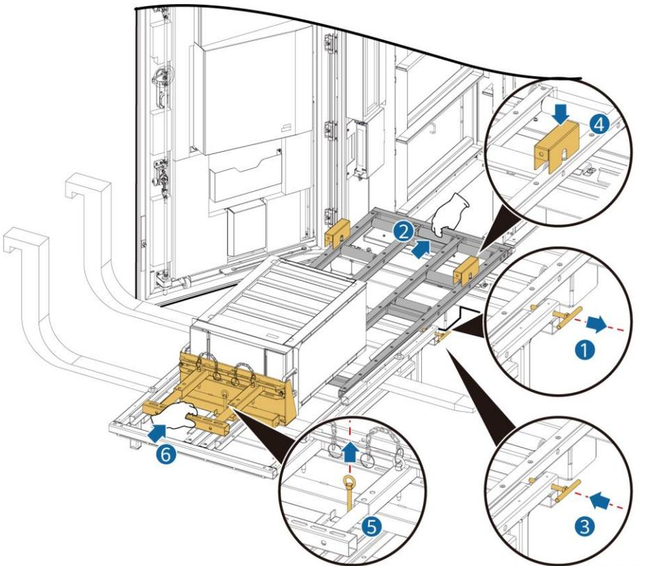
9. Move the battery pack into the installation slot.
