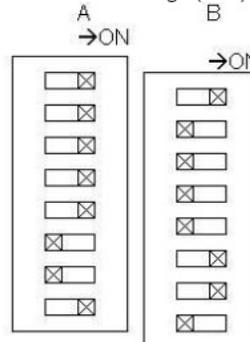
21 V low alarm on 23V alarm off
