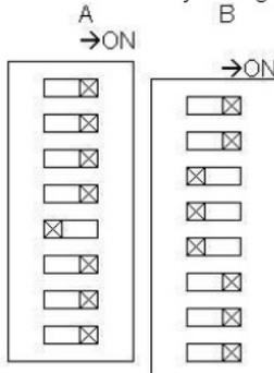
10.5V low alarm on 11.5V alarm off
