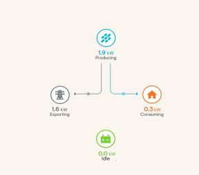
**Solar production** is powering the home, and because the batteries are fully charged, excess generation is exported to the grid.
