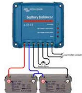
Battery Balancer (BM5012201000) The Battery Balancer equalizes the state of charge of two series connected 12V batteries, or of several parallel strings of series connected batteries. When the charge voltage of a 24V battery system increases to more than 27V, the Battery Balancer will turn on and compare the voltage over the two series connected batteries. The Battery Balancer will draw a current of up to 1A from the battery (or parallel connected batteries) with the highest voltage. The resulting charge current differential will ensure that all batteries will converge to the same state of charge.
