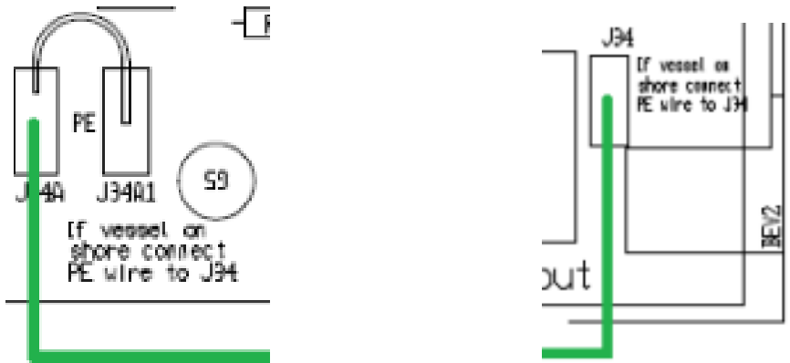
Figure 4a: Input earth connection, Auto 115/230V model
