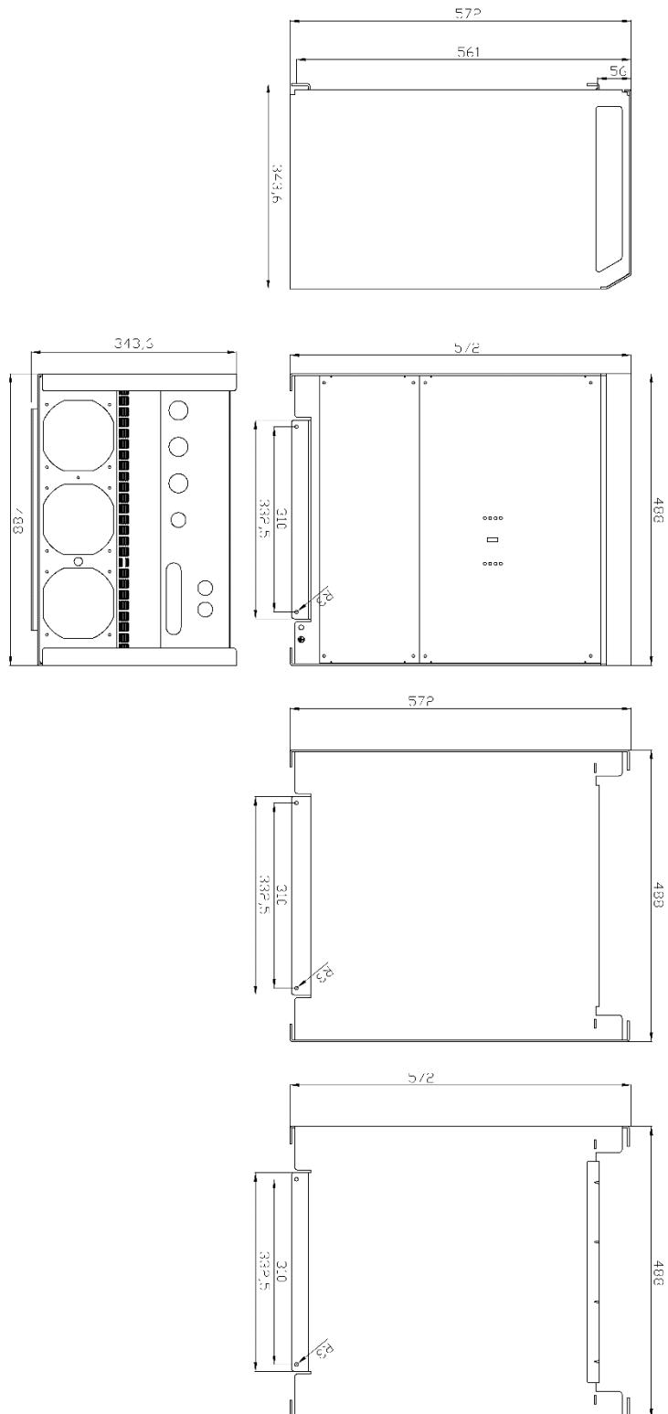
**Dimensions wall mounting plate Quattro 15kVA**
