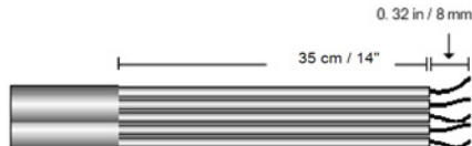
Figure 33: Insulation stripping – AC
