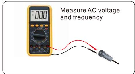
Step 2: Turn on the OCPD for the system and then measure the AC voltages line to line and line to neutral. The backup side of the system will be off until commissioning is complete. Turn the OCPD back off for now.
