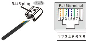
**Correspondence between the cables and the stitches of plug**
