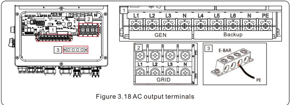
Figure 3.18 AC output terminals
