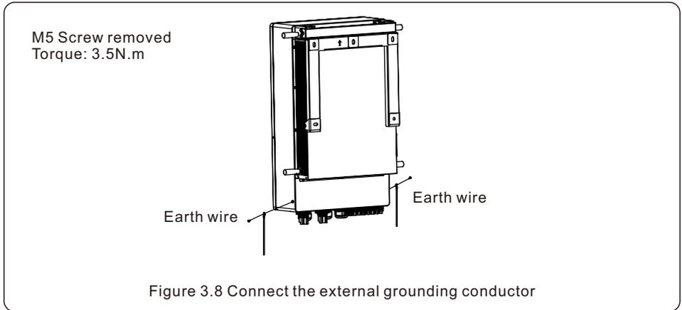
To connect the grounding terminal on the heat sink, please follow the steps below:
