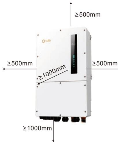
Figure 3.5 Inverter Mounting Clearances
