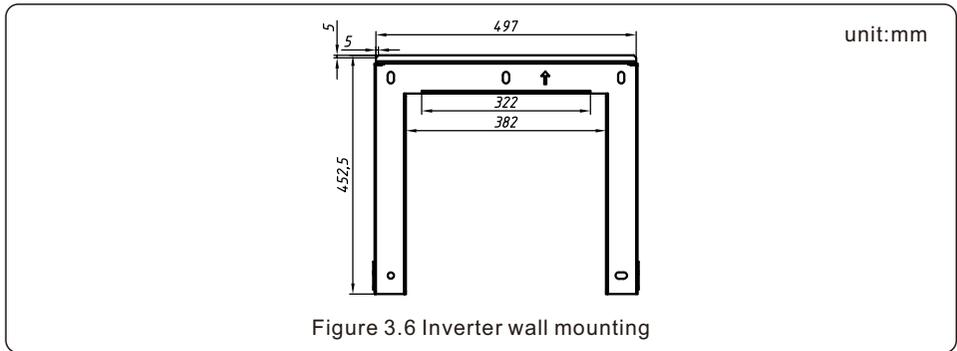
Once a suitable location has been found according to 3.1 using figure 3.6 mount the wall bracket to the wall.
