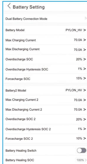
C. This type inverter allows you to connect two batteries, on quickly setting interface, we have a setting called “Dual Battery Connection Mode”, so when you connect the battery like 3.13 Lithium battery wiring (a), (b), you should choose the Battery independent selection, when you connect the battery like 3.13 Lithium battery wiring (c), you should choose the Battery in Parallel.
