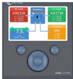
Color Control GX, showing a PV application
