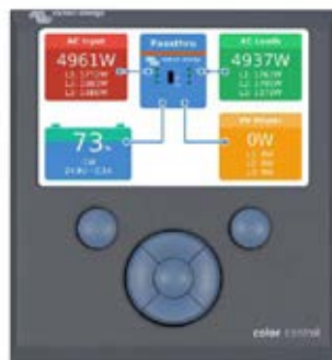
Color Control GX, showing a PV application
